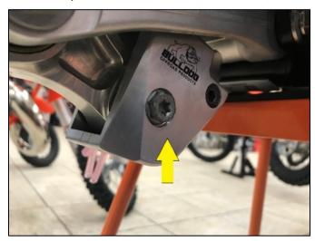
easier to remove the shock bolt. Remove the 13mm bolt from the rear suspension shock on the right-hand side of the motorcycle. Be careful, the rear wheel will drop to the ground and the shock mount will be loose as well.
